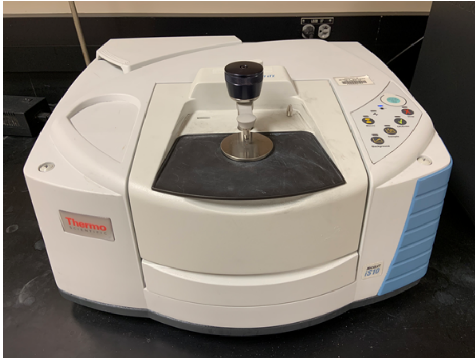
Figure 10: Thermo Scientific Nicolet iS10 FTIR device with Smart iTX accessory.
