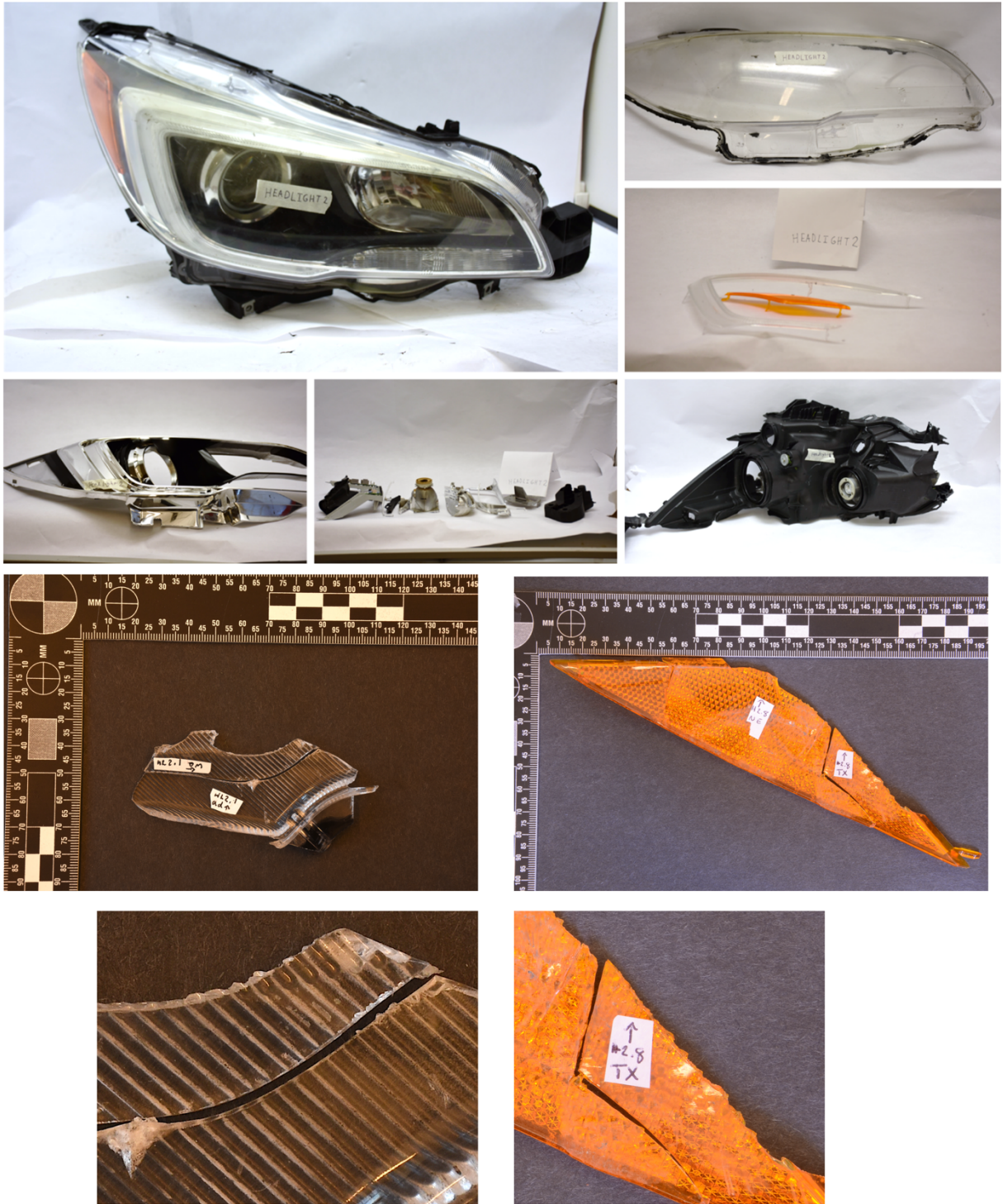
Figure 16. Images of an original headlight and the separated components before fracture. The initial assembly is shown in the top left image. The lamp is taken apart to separate the different types of polymers and remove non-polymer parts (metal/glass). The bottom four images are examples of reassembled and relabeled true-fit pairs for the clear and orange portions of the headlight, and a zoomed image of the edges, respectively.
