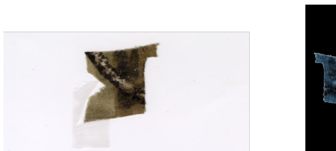
Figure 12. Example input of a textile image. This image shows one side of the textile. One of the edges has been cut in a triangle shape, representing a non-comparison edge. The preprocessing reduced the original image to the two edges, and the non-comparison edge will not be used.
