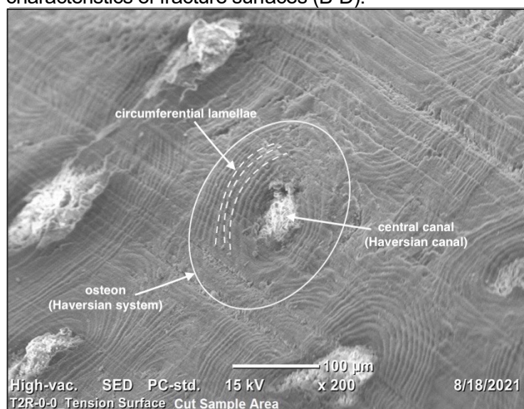
(A) Osteons visible on a cut surface of bone. Magnification=200X. These osteons lack pullout, delamination, and microfractures.
