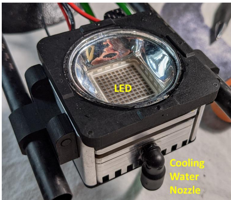
Figure 120. LED unit of Illuminir reader design showing a cooling water inlet.
