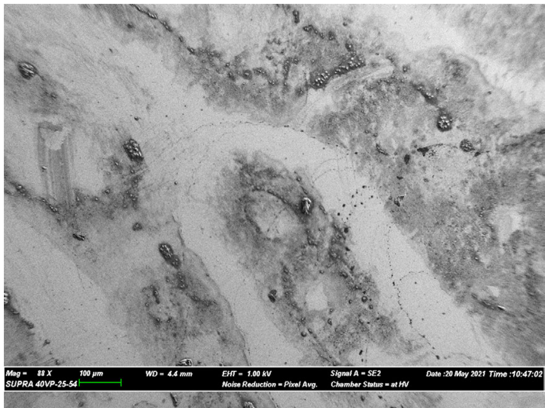
Figure 89. Undeveloped fingerprint on silicon after a five second toluene rinse. SEM image taken at 1 kV and 88x magnification. Some crystals are observed on this image. In addition, the area between the ridges is much clearer after rinsing in toluene.
