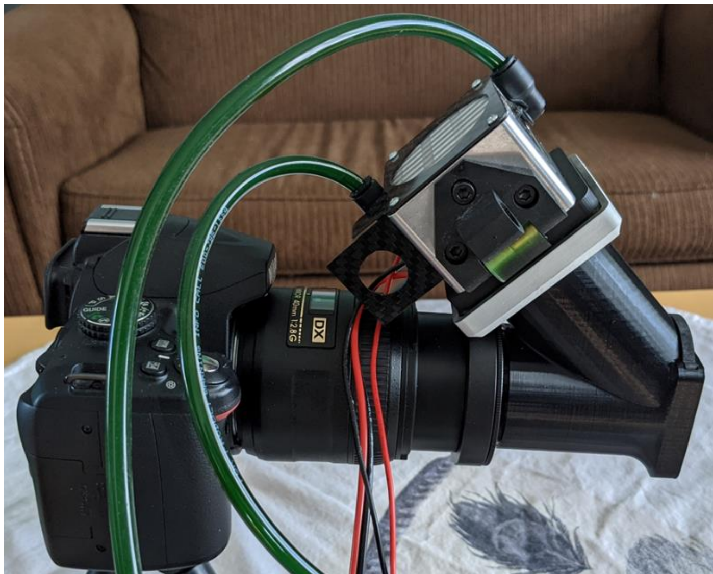
Figure 127. Camera mount connecting the LED unit to the camera.
