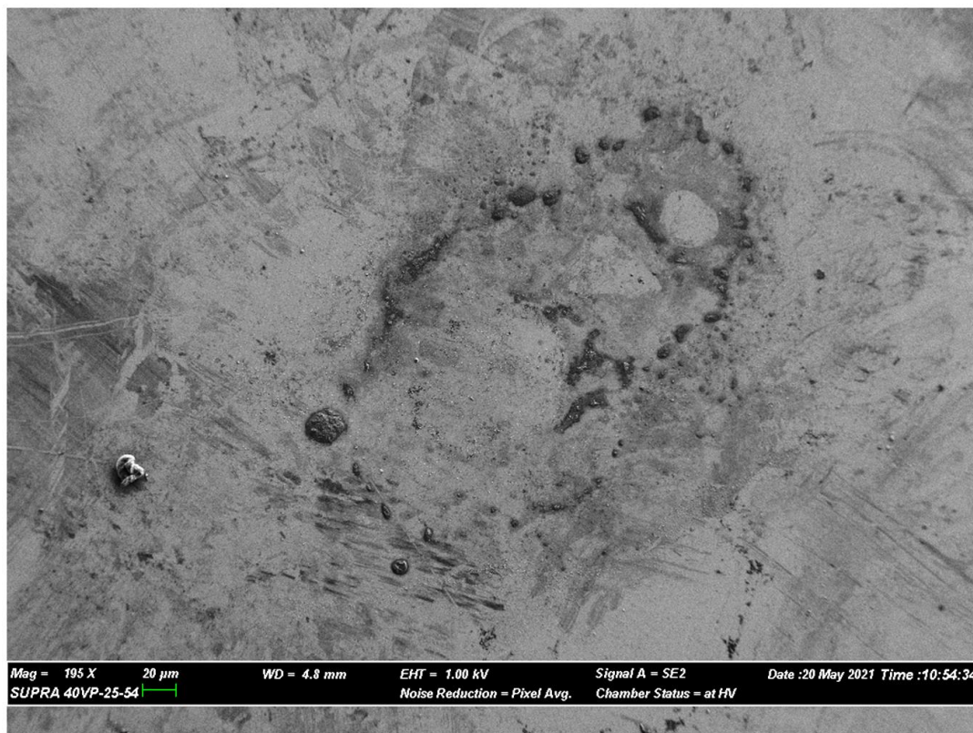
Figure 91. Undeveloped fingerprint after Sono-tek treatment and toluene rinse at one kV. The low voltage used allows greater surface sensitivity and much excess material can be observed here.
