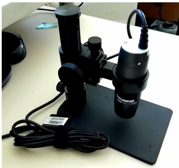
Figure 20. Dino-Lite fluorescent digital microscope equipped with an emission filter of 510 nm and a blue LED excitation light source (480 nm) was used to visualize the presence of dyed material.
