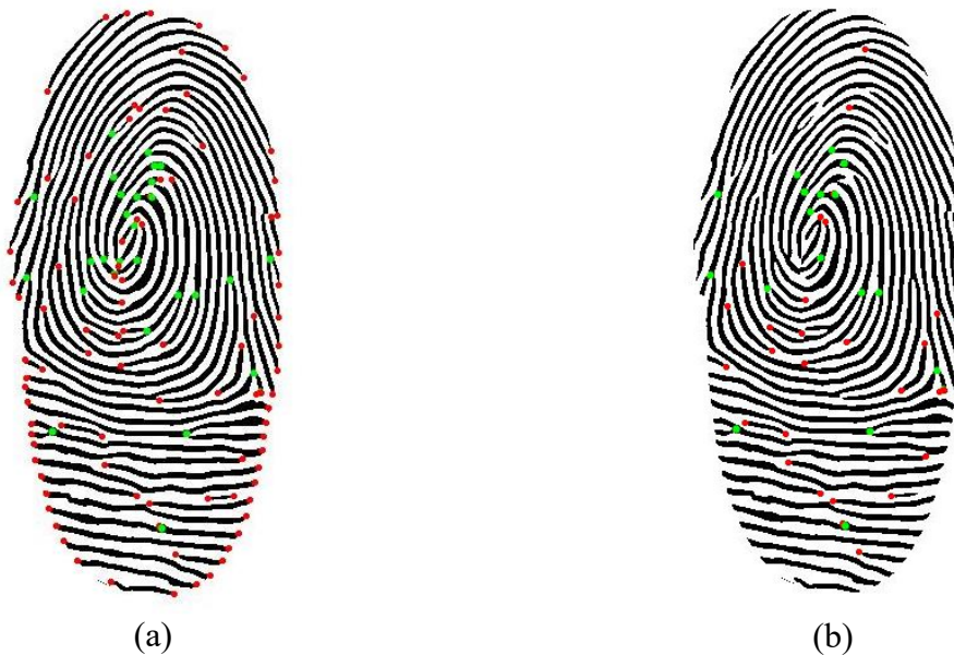
Figure 96. Extracted minutiae (a) before CNN verification (b) after CNN verification.
