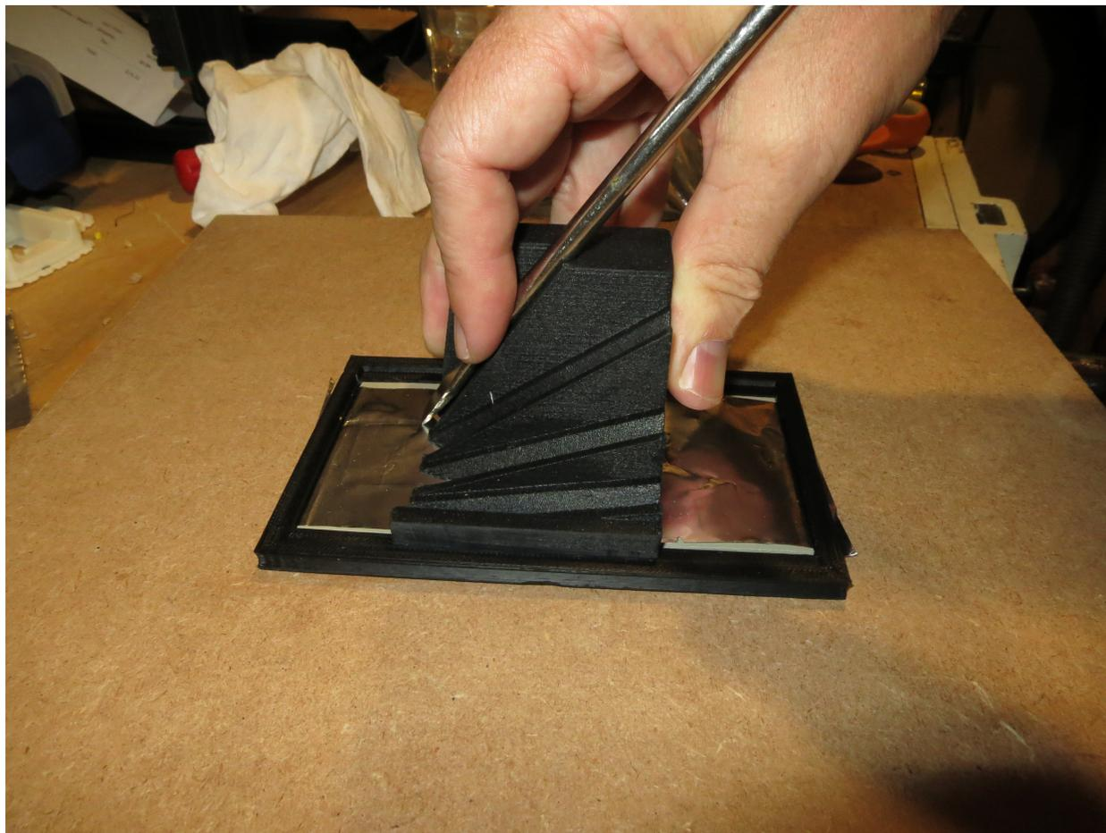
Figure 13. Custom 3D printed Jig for making toolmark impressions.
