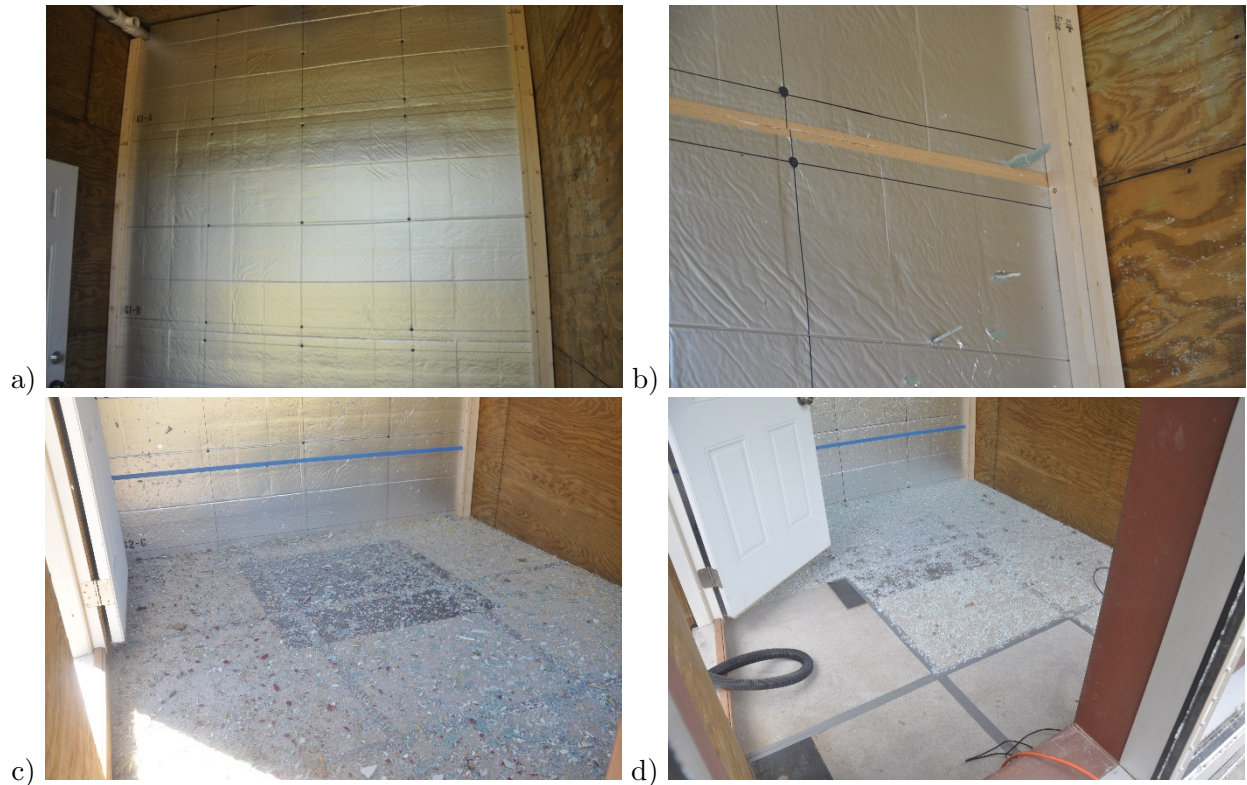
Figure A2. Additional test protocol for glass specimens: a) use of an ASTM F1642-12 witness panel at the rear of the test enclosure to document high hazard glass debris; b) photograph of glass debris captured by witness panel; c) glass debris on floor across nine demarcated areas; d) collection of glass debris from demarcated areas to quantify the distribution of mass of glass debris throughout the enclosure
