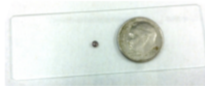
Fig. 1. SERS Au nanoparticle covered chip (2 mm) on a glass slide compared with dime.
