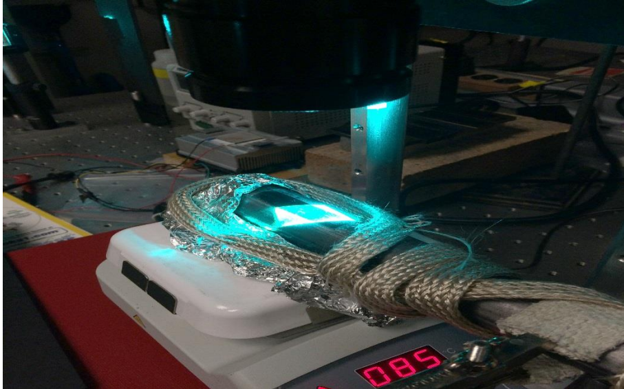
Figure 52 Defaced gun barrel mounted on the constant temperature hot plate in the thermal imaging experiment.
