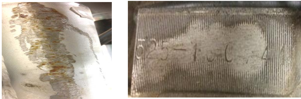
Figure 56 Defaced VIN number and defaced motor ID number from Yamaha motorcycle.
