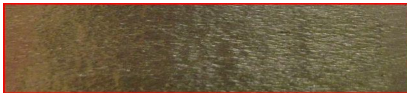
Figure 16 Photographic image of a defaced unfiltered aluminum test sample of the defaced serial number 22789043.
