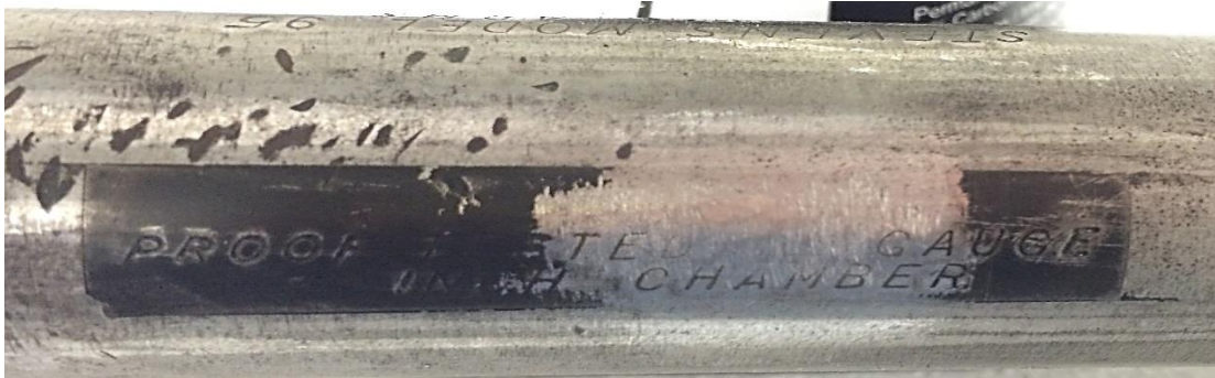
Figure 51 Picture of the gun barrel after defacing the 1 and 2 from the label "12 gauge".
