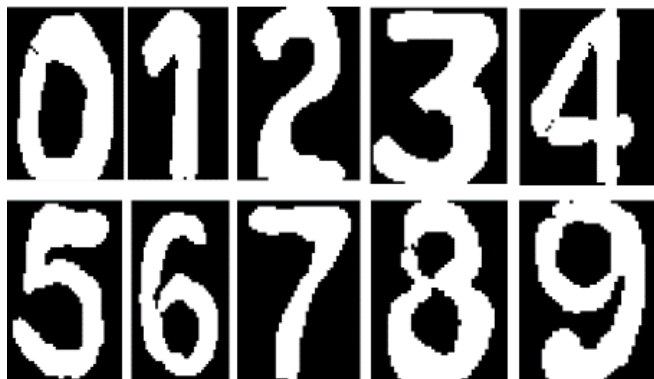
Figure 45 Library 2 of number digits 0-9. This is a modification of Library 1 to account for the expected broadening in the numbers in the plastic deformation region.
