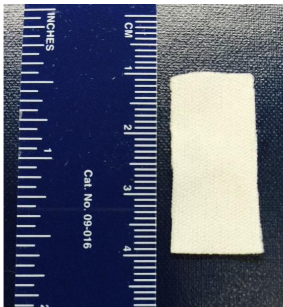
Figure 3.2 Cut CapSure® VP swab measuring approx. 3 x 1.5 cm used as sampling media.
