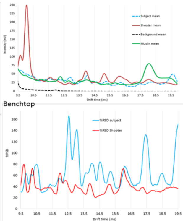
Figure 2.10 Summarized results for authentic samples analysed with the Ionscan® (benchtop) instrument.
