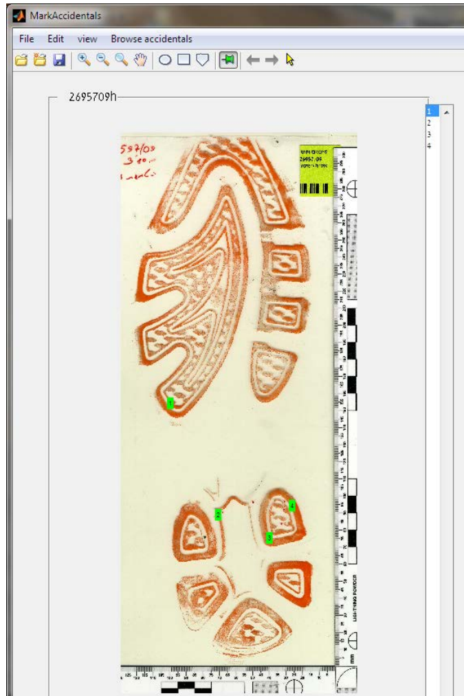
Fig. 4. Location of already marked accidentals and their ID numbers shown over the test impression.
