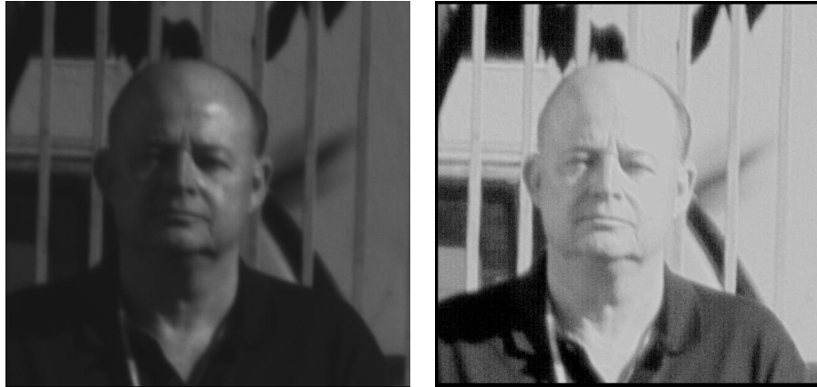
FIG. 16 Dynamic range compression: (a) original image; (b) luminance enhanced image processed via dynamic range compression.
