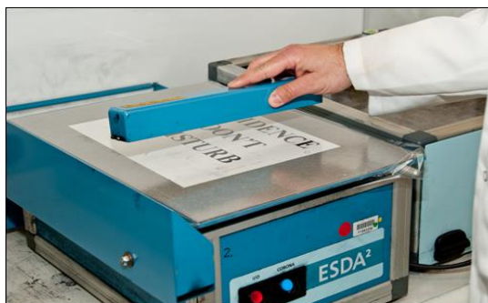
Figure 2: Collection of indented writing in a sample document using an ESDA [7].
