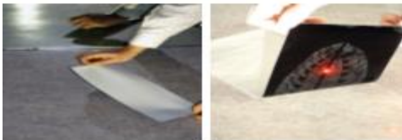
Figure 7: Collection of a latent shoeprint using BVDA gelatin lifters.
