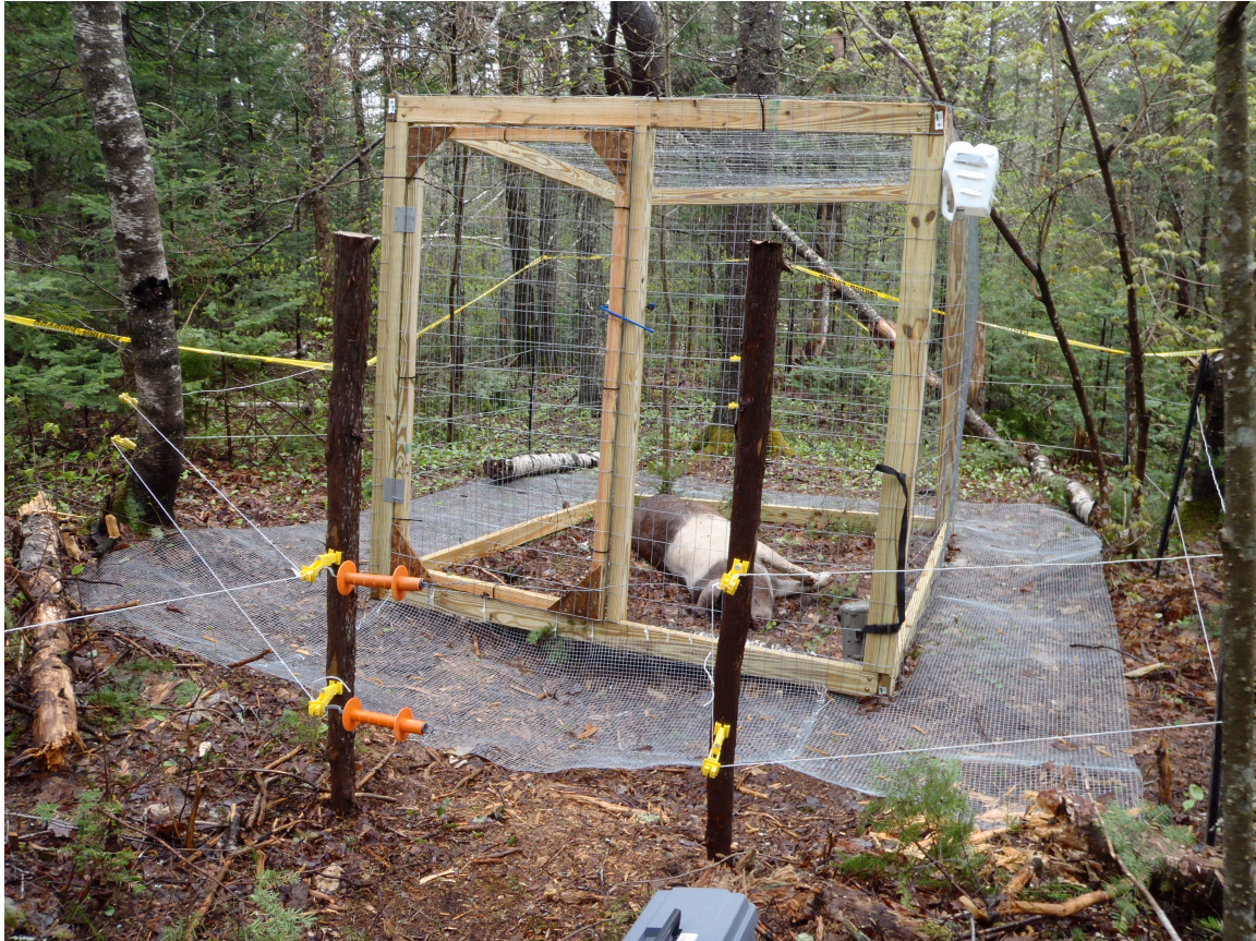
Figure 6. Example of a caged pig located in a mixed deciduous-evergreen woods. Cage has a 3-foot skirt surrounding the cage to prevent access by burrowing animals. Two cameras are present, one inside and one outside the cage. An electrical fence surrounds the site. The white temperature and humidity data logger housing is at the top right of this image.
