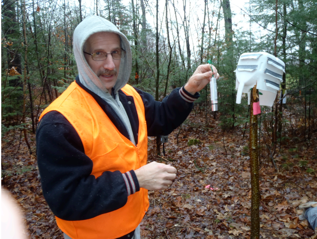
Figure 1. Temperature and humidity data logger and white plastic, ventilated housing and solar shield
