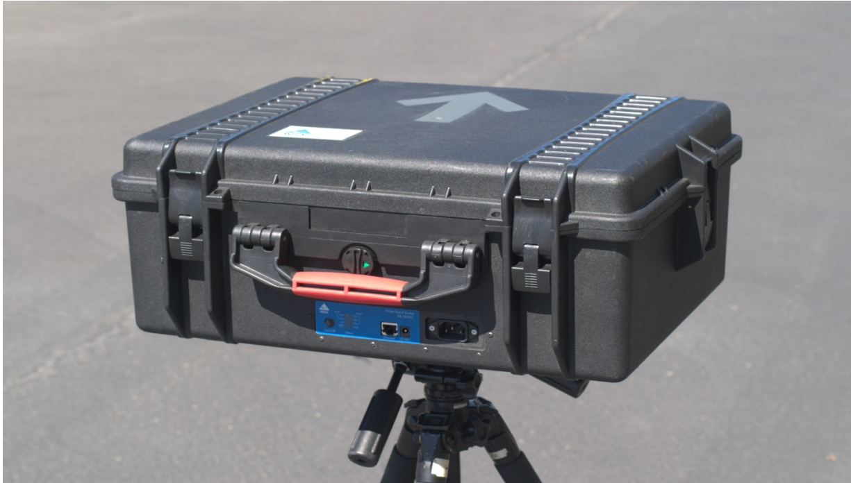
Figure 1 ASTIR (AKELA Standoff Through the Wall Imaging Radar) system
