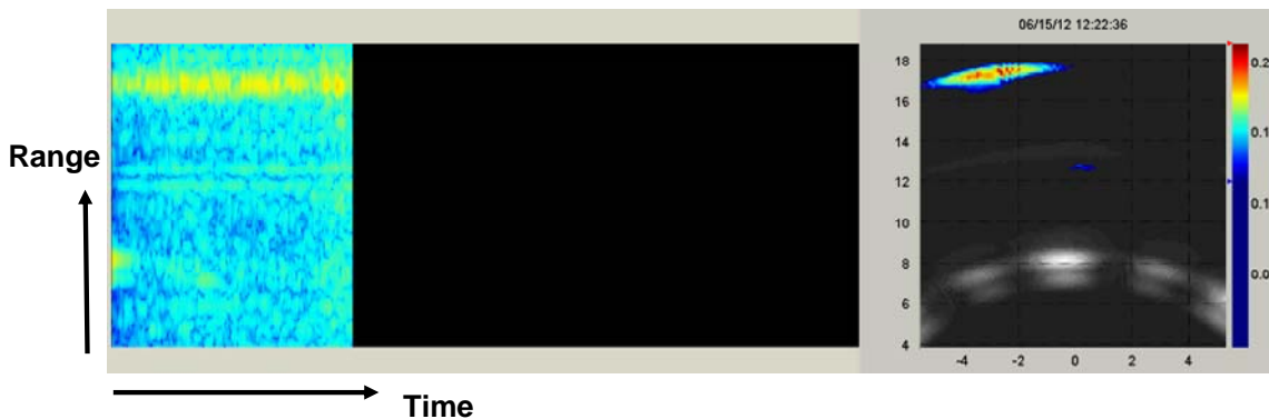
Figure 14 – Successful detection of stationary individual through two walls
