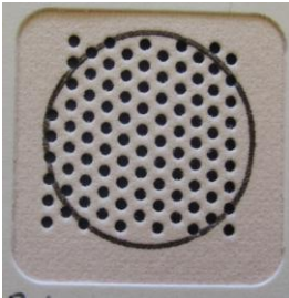
Figure 10. EasiCollect card that has been punched 96 times using the automated system. The punches have a diameter of 1.2mm.
