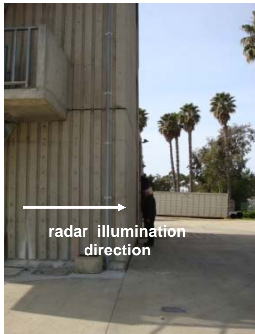
Figure 20 Stationary Human Detection Through 0.53 m of Steel Reinforced Concrete
