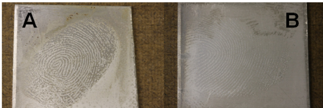
Figure 13. Fingerprint ridge detail photographed after being treated for 24 hours with Tek Gel™; (A) finger coated with oils from forehead swipe and (B) finger not coated with oils.
