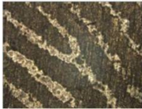
Figure 3. Microscopic digital image examining the bare metal protected by fingerprint oils versus acid-vapor corroded bare material
