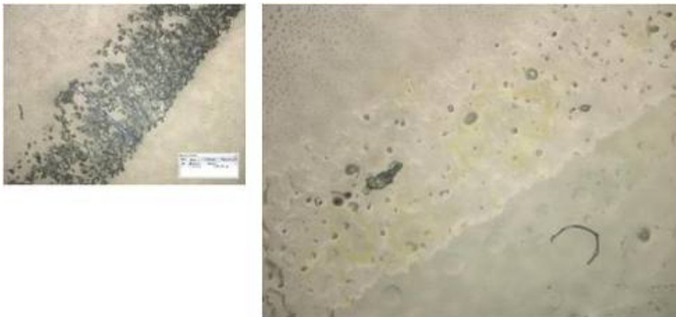
Figure 16. Phenolic resin dissolution in organic solvent vapors occurs extremely rapidly. The small image is phenolic resin particles dusted onto calibrated oil lines
