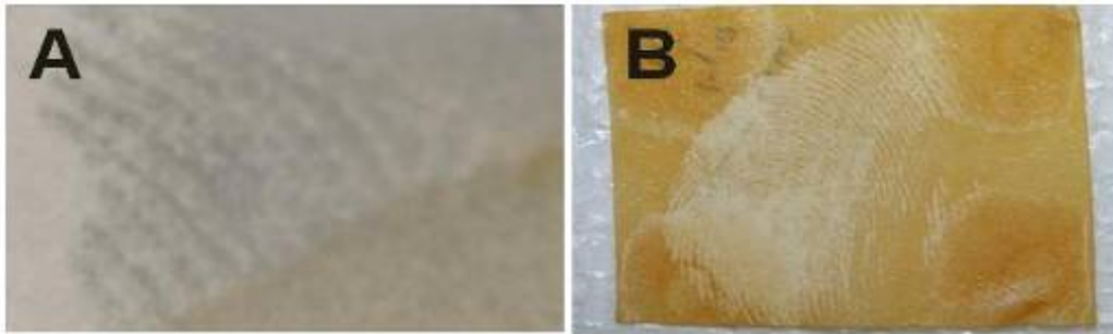
Figure 4. Digital photographs (A) before and (B) after exposure to iron salt solution
