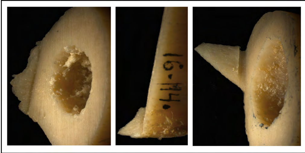
Figure IV-5. Three examples of break-away spurs. Photographs taken of bone sections created for previous NIJ funded research grant.
