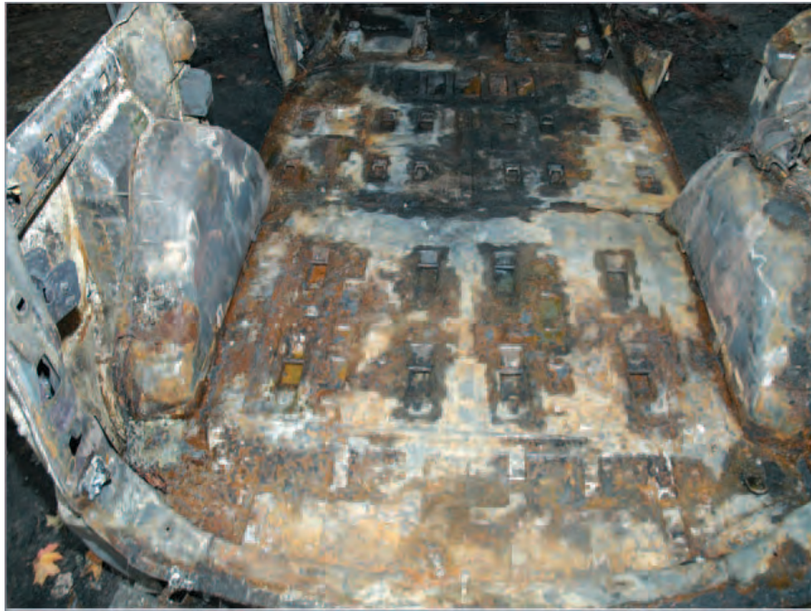
Figure II-23. Interior view of vehicle following excavation in which all debris, evidence, and human remains were removed.
