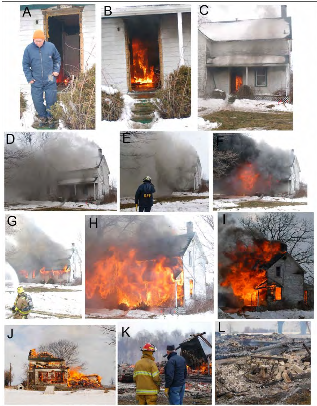
Figure 4. Fire progression. (A-C) Initial ignition of structure with a road flare. (D-E) Within minutes of ignition. Temperature readings being taken (E). (G-I) Fire progression. (J-L) In a little over two hours all walls of the structure had collapsed and the structure had burned to the ground.
