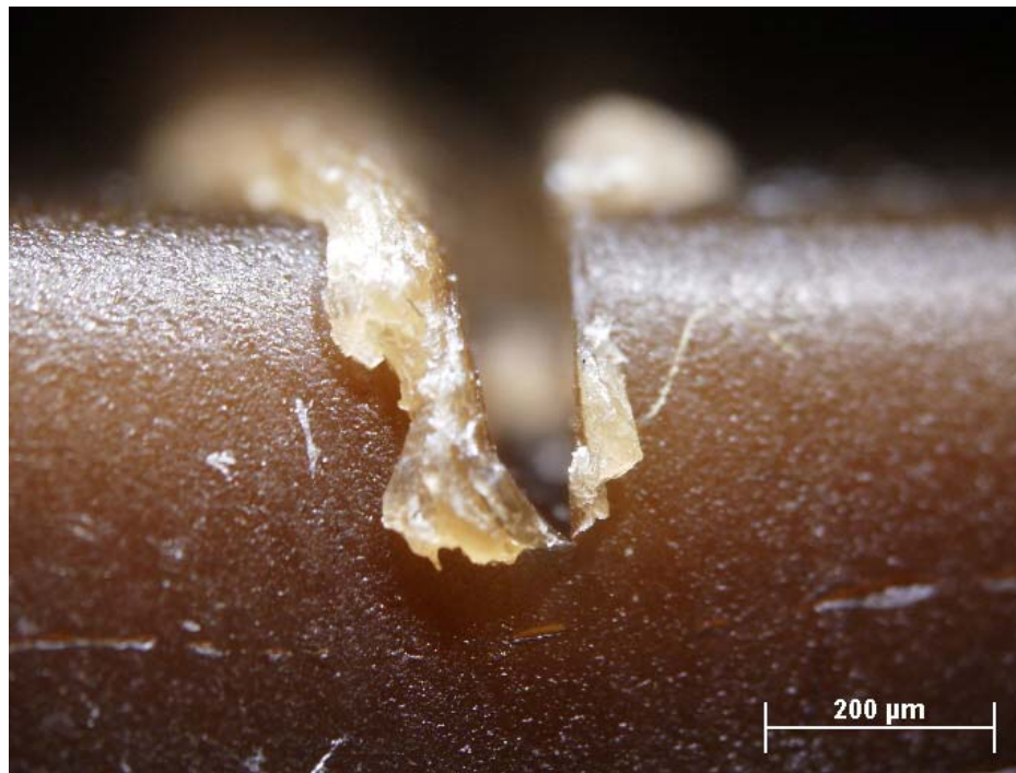
Figure 5. 20x image showing kerf shape indicating a left edge bevel.
