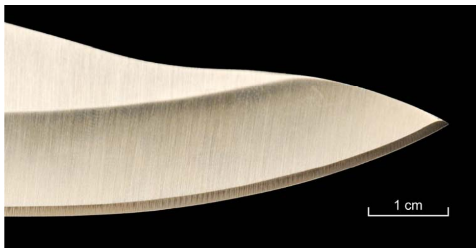
Figure 9. The surface of one of the non-serrated blades misclassified as a serrated blade. Note the distinct pattern left by the milling of the beveled edge.
