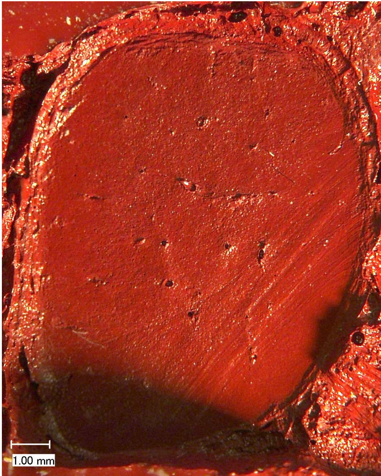
Figure 11. View (20x) of the opposite kerf wall shown in Figure 9. It is important to examine both kerf walls.
