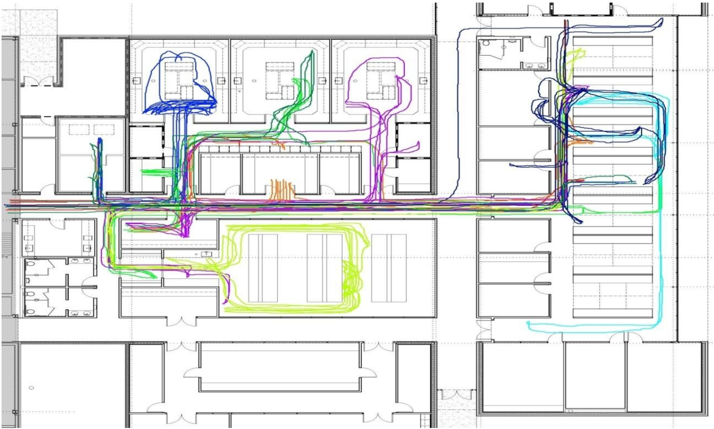
Figure 16: Current state spaghetti chart of a simple blood-only evidence case. A total of 8,808 feet (1.67 miles) were traveled to complete processing this case. Each different color represents a different step of the process.
