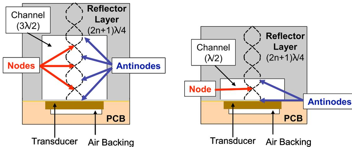
Figure 3: Schematics of the channel design such that acoustic resonators are constructed and standing waves are obtained in the microchannel. *Right.* Single node microchannel: the depth of the channel is  $1/2$  wavelength ( $\lambda$ ) and the thickness of the reflector layer is  $5\lambda/4$ . *b. Left.* Triple node microchannel: the depth of the channel is  $3\lambda/2$  and the thickness of the reflector layer is  $3\lambda/4$ . Note: drawings are not to scale.
