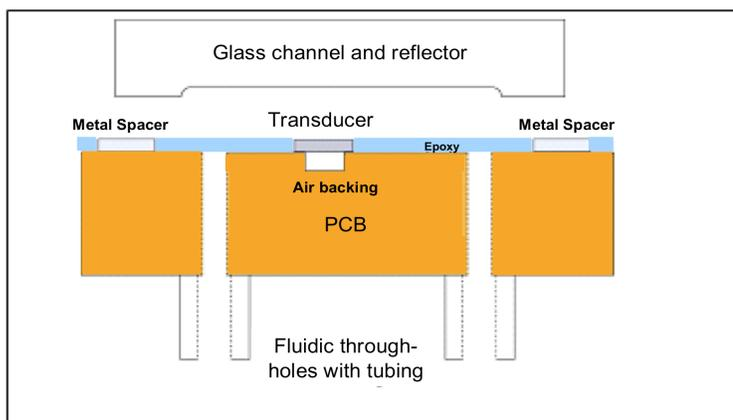
Figure 1: The ADE Microdevice. *Left.* A schematic image showing the components of the ADE system with the PCB holding the transducers and the fluidic access and a separate glass-chip, defining the microfluidic network. *Lower Left.* The device consists of b. a printed circuit board containing piezoceramic transducers, and a fluidic layer (reflector layer) composed of borosilicate glass. *Lower right.* Sealed ADE microdevice in a brass interface.
