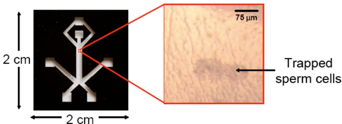
Figure 5: Channel structure of microdevice with the location of the transducer outlined in red. Inset: Photomicrograph of spermatazoa trapped above a microtransducer.
