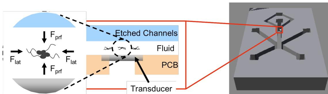
Figure 4: ADE device schematic. Inset: cross-sectional view of the device from the area above the transducer. Sperm cells are shown trapped above the transducer by primary ( $F_{prf}$ ) and lateral ( $F_{lat}$ ) forces at the node of the ultrasonic standing wave.
