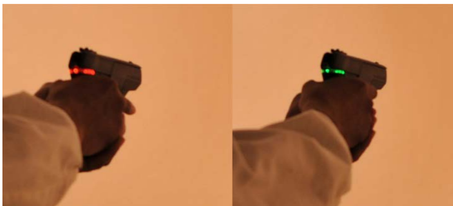
Figure 14. Indicator lights on the iP1 showing the firearm in an unauthorized state (red) and an authorized state (green) during a test firing of the Smart System at the Maryland State Police Forensic Science Laboratory in February 2013. Permission to use images granted by Maryland State Police Forensic Science Laboratory.
