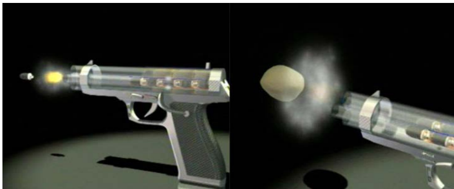
Figure 10. Computer visualization showing the ammunition stacked in line. A lethal round can be fired (left) or a nonlethal round can be selected (right). Stills from a video submitted by Metal Storm to NIJ that demonstrate the functionality of the prototype designs.
