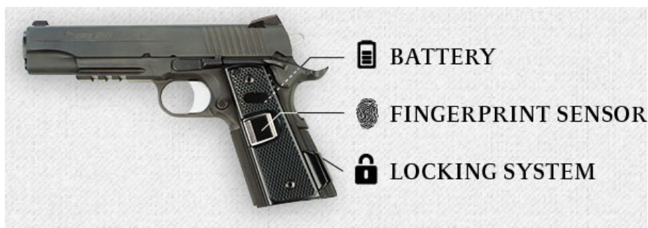
Figure 17. Intelligun system featured on a model 1911-style pistol (from reference 103).
