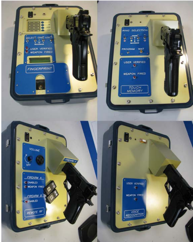
Figure 1. Various demonstrators produced by Sandia National Laboratories to illustrate the basic functionality of user authorization technologies, such as fingerprint (upper left), touch memory (upper right), remote RF (lower left), and voice recognition (lower right).
