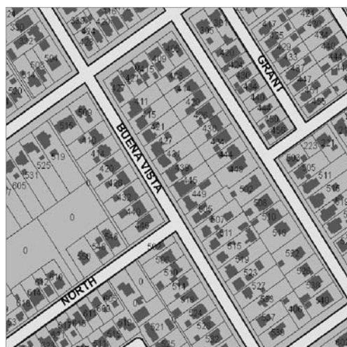
Figure 2. 1:50000 scale. All streets are labeled and symbolized equally. Building outlines and parcels are visible. Address numbers are labeled.
