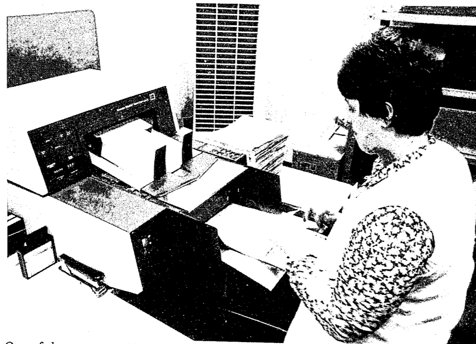
One of the new microfilm cameras provided for processing accident record information in Traffic Division.
