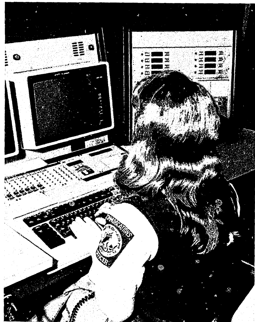
The field service console has greater radio capability and a high-speed projector for sectional maps.
