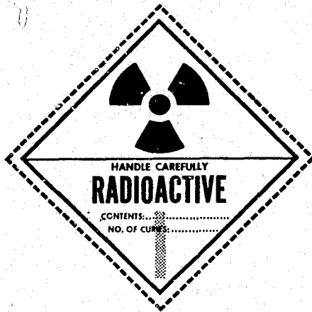
"Radioactive white-I" label for radioactive materials. Label must be white in color. The single vertical bar on the lower half of the label must be bright red in color.
