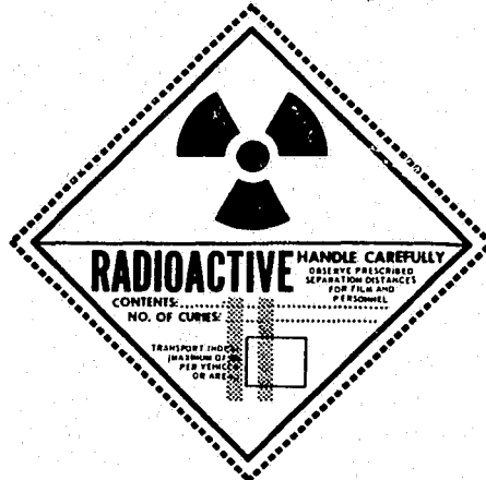
"Radioactive yellow-II" label for radioactive materials. The upper half of the label must be bright yellow and the bottom half must be white. Two vertical bars on the lower half of the label must be bright red in color.
