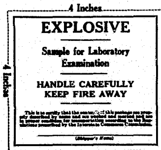
RED LABEL FOR SAMPLES OF EXPLOSIVES (Reduced size) (Black printing on red)
