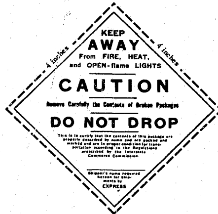
YELLOW LABEL FOR FLAMMABLE SOLIDS AND OXIDIZING MATERIALS (Reduced size) (Black printing on yellow)
