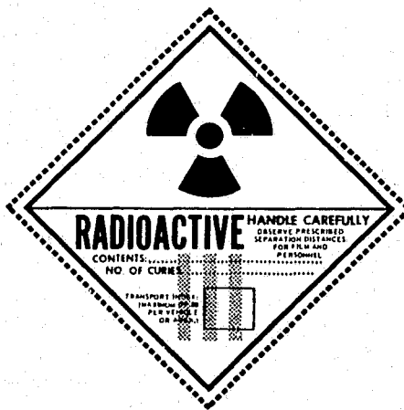
"Radioactive yellow-III" label for radioactive materials. The upper half of the label must be bright yellow and the bottom half must be white. The three vertical bars on the lower half of the label must be bright red in color.
