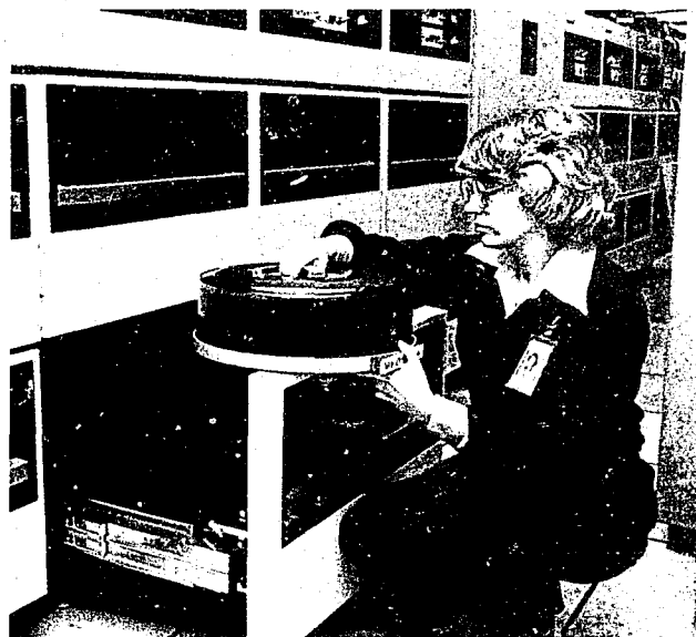
Computer operator prepares to load data base information on new disk system. Disk shown holds 94.5 million characters of information.
