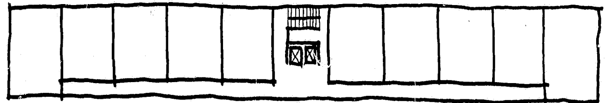
Figure 3.21: Typical plan of single-loaded corridor high-rise building.
