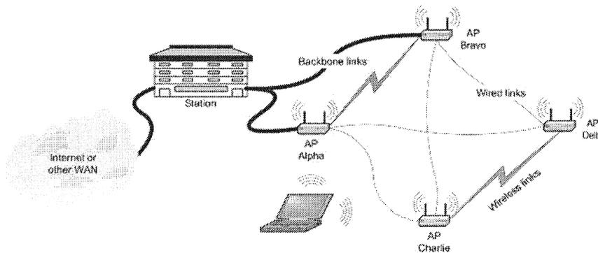
**Figure 17-2: Mesh Networking of WLAN Access Points**
