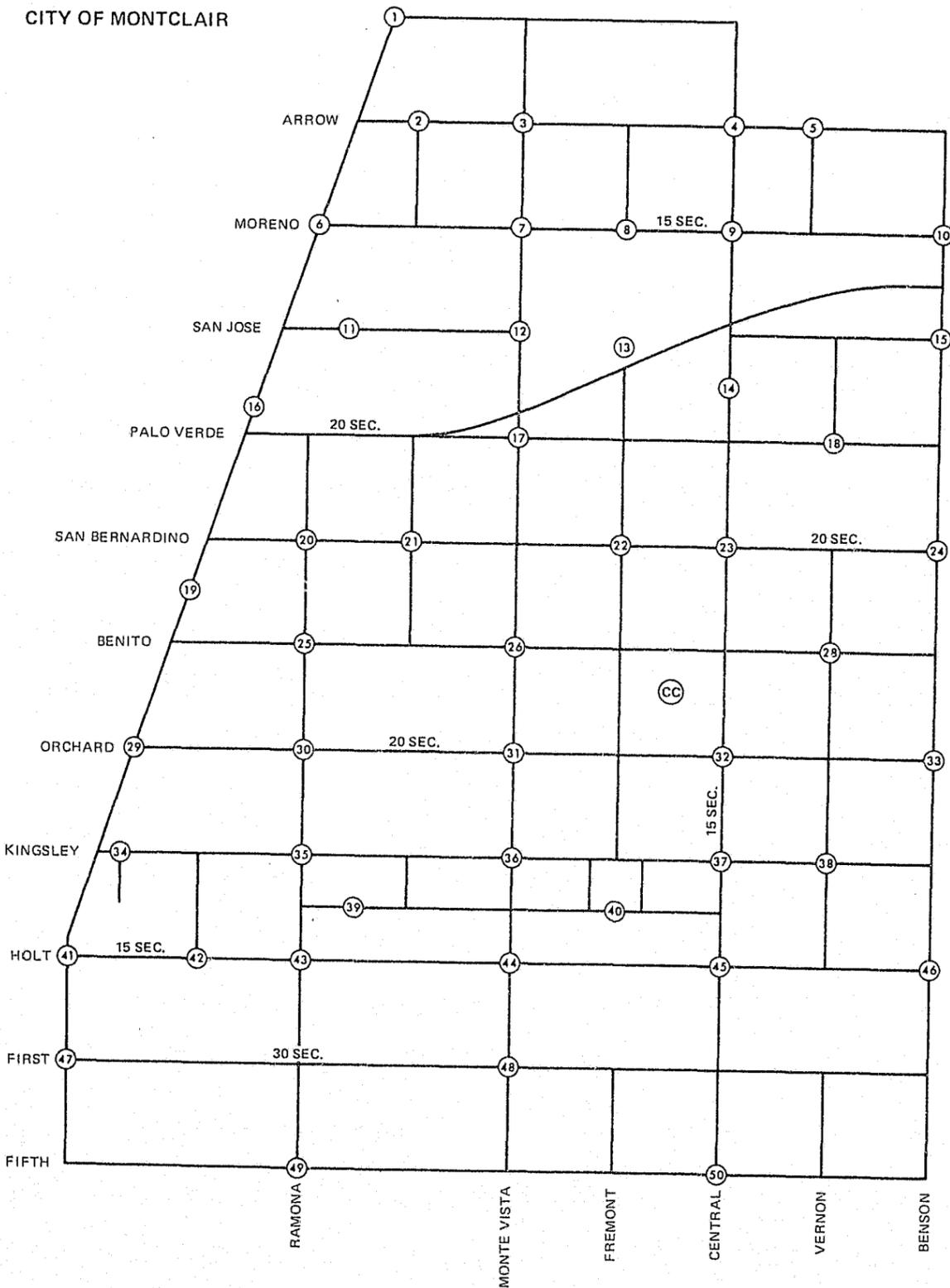
Figure 7. Placement Of Wayside Emitters In Montclair
