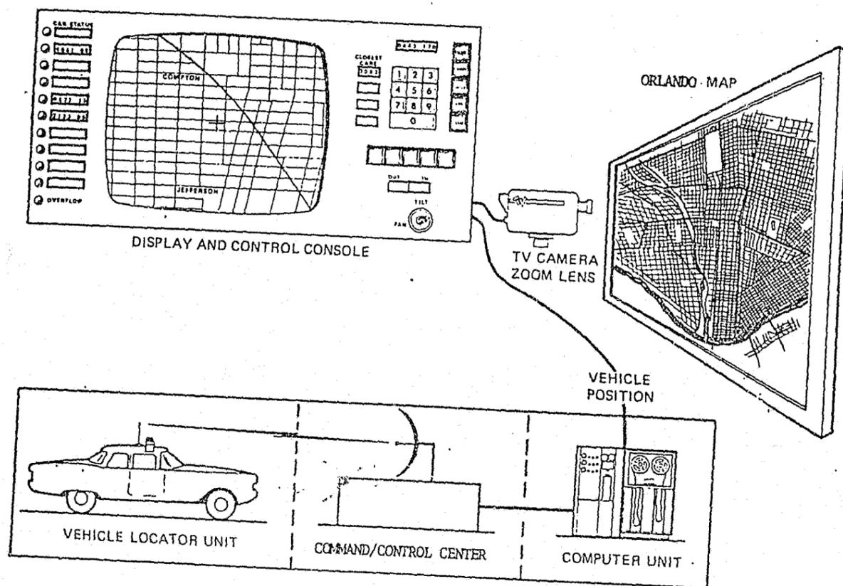
Figure 6: FLAIR System Concept Shows Major Functional Components and their Interrelationship
