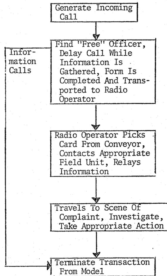
Figure 2. The comparison of GPSS/360 Program Logic Blocks to Flow Chart of actual system.
