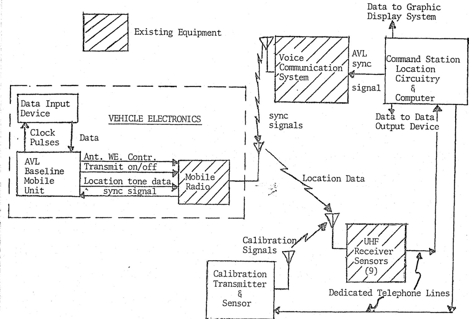
Figure 5: AVL System Block Diagram Shows Compatibility with Existing PREP System
