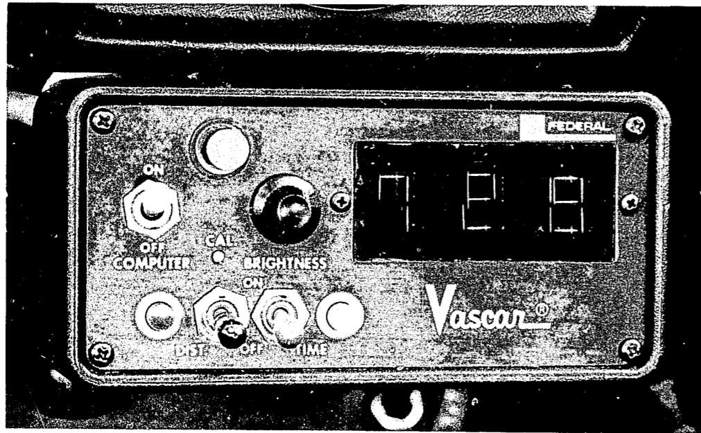
The VASCAR (Visual Average Speed Computer and Recorder) as fitted in a police car
