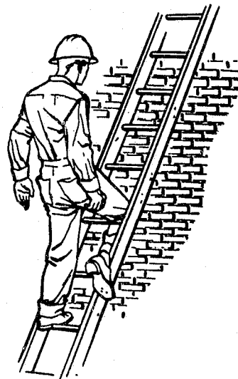
FIGURE 26.—Ladder leg lock.
